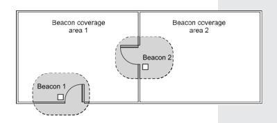
Beacons are installed next to doors, gates or other points of interest. Their coverage is minimized (with power adjustment) to track subscriber entering/exiting proximity with greater accuracy.
