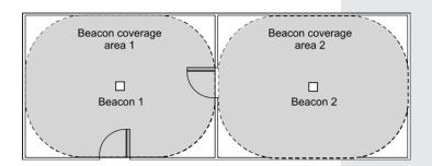
Each beacon is installed in the center of a room and completely covers it. For large rooms and halls, multiple beacons are installed in the way that their coverage areas are not overlapping. For this, beacon power is adjusted and their placement is determined with respect to that purpose.
